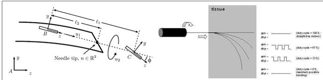
Configuration of bicycle model parameters during insertion of flexible bevel tip needle(left) and duty cycle-controlled needle steering (right)
