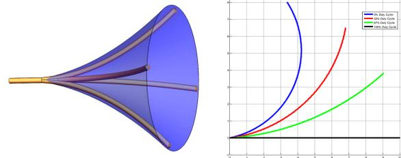
Needle steering in four directions of 3D space within the cone bounded by the maximum curvature (left) and simulated trajectory of a flexible bevel tip needle at various duty cycles (right).
