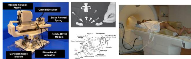
6-DOF piezoelectric actuated needle placement robot (left); fiducial frame and rotary motor fixture, an exploded view of the needle clamping mechanism (middle); mockup test of human inside MRI (right)
