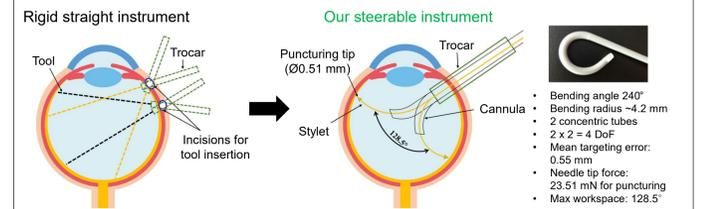
Leveraging our ultra-steerable instruments, our eye surgery robot can provide a safer and less invasive procedure with a larger workspace
