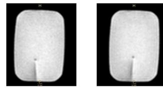
Example of needle trajectory control by steering the needle during insertion under real time imaging using the orientation of the bevel tip
